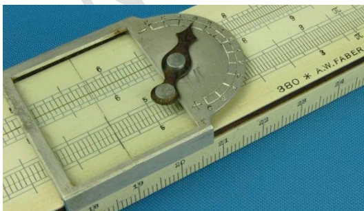
Figure 2: Faber 380 with digit registering cursor
