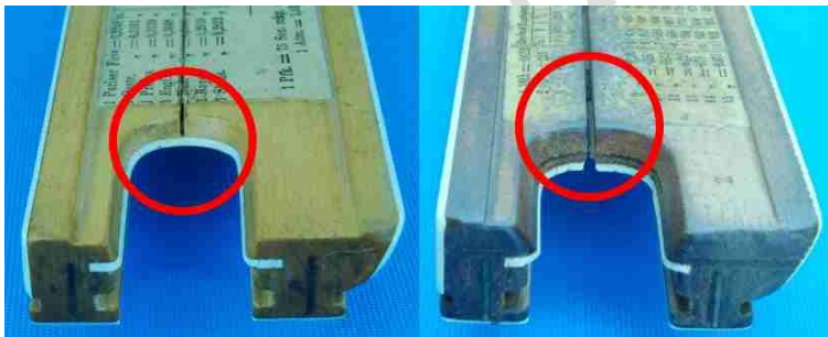
Figure 4: 2-part celluloid-sprung stock (left) and 2-part steel-sprung stock (right).
